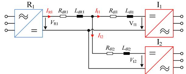
Fig. 4: Basic scheme of a three terminal system
