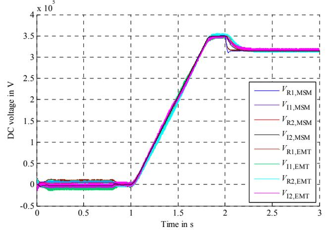
Fig. 14: DC voltages of the MT HVDC models
