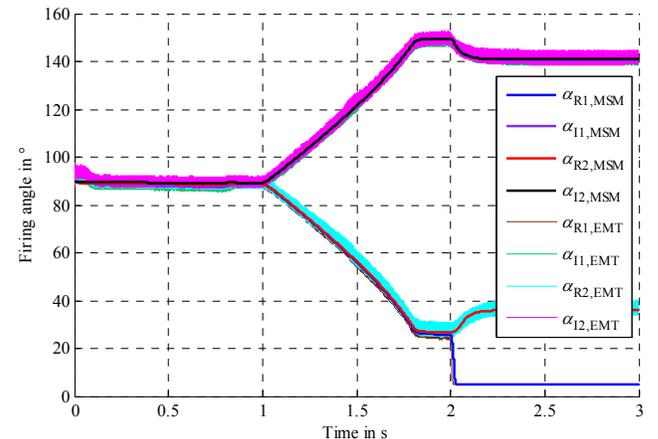
Fig. 15: Firing angles of the MT HVDC models
