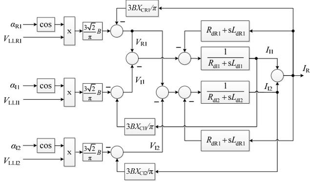
Fig. 5: Block diagram of a three terminal HVDC system
