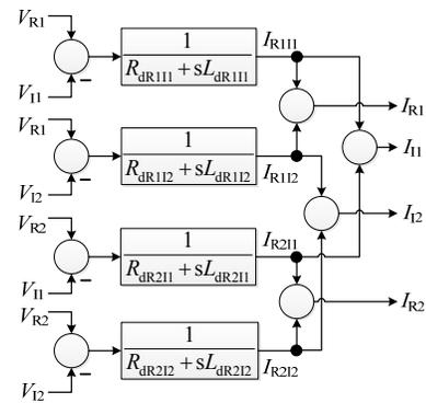
Fig. 8: Superposition of partial DC currents in a four terminal system
