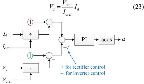
Fig. 11: CCCM control scheme at rectifier and Inverter respectively
