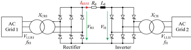
Fig. 2: Schematic layout of a six-pulse point-to-point HVDC system
