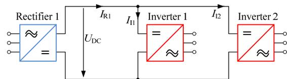
Fig. 1: Basic scheme of a three terminal parallel HVDC converter arrangement
