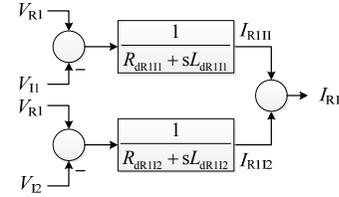
Fig. 7: Superposition of partial DC currents in a three terminal system
