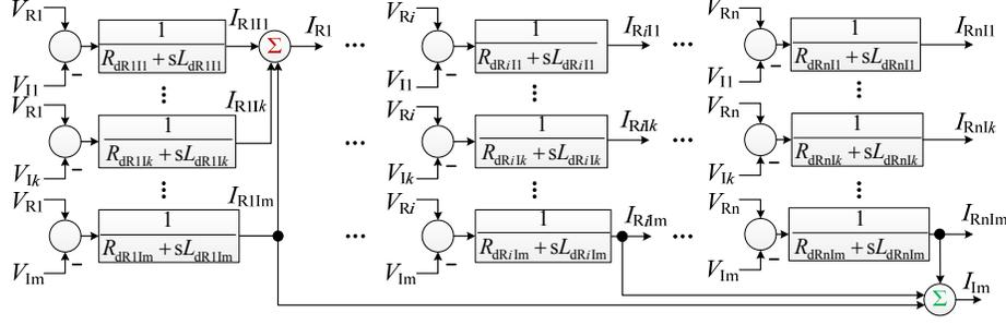
Fig. 9: Block diagram of a Multi-Terminal system with superposition of partial currents
