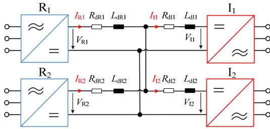
Fig. 6: Basic scheme of a four terminal system
