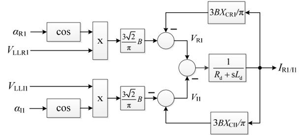
Fig. 3: Block diagram of a point-to-point HVDC system
