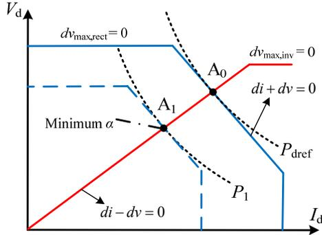
Fig. 12: Adjustment of the V-I-characteristic of the CCCM during an AC voltage drop at a rectifier
