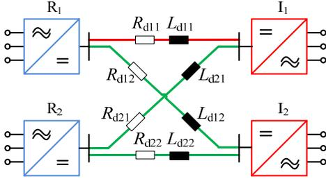
Fig. 10: Basic scheme of a meshed four terminal system
