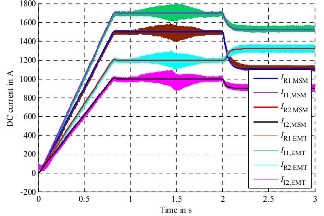
Fig. 13: DC currents of the MT HVDC models
