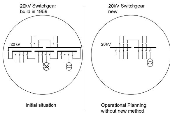
**Figure 2: Switchgear configuration of the existing system and after operative planning**
