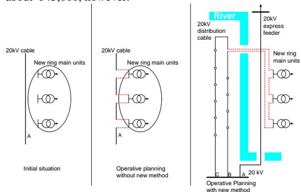
**Figure 4: connection of three ring main units**
