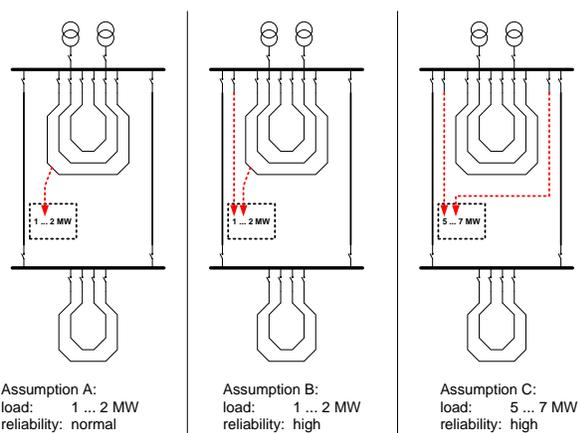
Figure 6: Network configurations for different load scenarios
